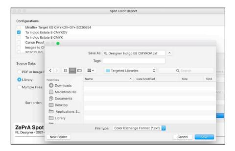
**Below:** The ZePrA **Spot Color Report**'s exported Lab library can be imported and used in handheld instruments or process control software so that measured results can be weighed against expected values of spot color simulations calculated by ZePrA and approved by customers. In this case deltaE numbers suddenly become simple and meaningful.
